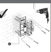
When selecting the position of the TV mount. ensuring that the mount will be mounted on to a flat surface and is level. Mark the wall where the fixing locations are. Drill the holes using a 10mm masonry bit. Using a hammer knock the the wall plugs (C) provided into the wall. Holding the TV mount start in the one corner screw the provided screws (B) into the wall fixing the opposite corners until the mount is secure onto the wall. Ensure all are tight and secure.
