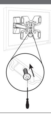
Using a screwdriver tighten the securing bolts onto the mount.
