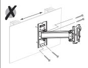
Ensure that the mount is fixed to a solid object and not into plasterboard on its own.
