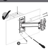
Using the provided self taping screws (B) type. Holding the TV mount starting in the one corner, screw the provided screws (B) into a wooden joist fixing the opposite corners, until the mount is secure onto the wall. Ensure all are tight and secure.
