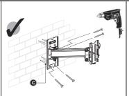
When selecting the position of the TV mount. ensuring that the mount will be mounted on to a flat surface and is level. Mark the wall where the fixing locations are. Drill the holes using a 10mm masonry bit. Using a hammer knock the the wall plugs (C) provided into the wall. Holding the TV mount start in the one corner screw the provided screws (B) into the wall fixing the opposite corners until the mount is secure onto the wall. Ensure all are tight and secure.
