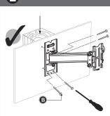
Using the provided self taping screws (B) type. Holding the TV mount starting in the one corner, screw the provided screws (B) into a wooden joist fixing the opposite corners, until the mount is secure onto the wall. Ensure all are tight and secure.
