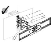
Using the provided self taping screws B type). Holding the TV mount starting in the one corner, screw the provided screws (B) into a wooden joist fixing the opposite corners, until the mount is secure onto the wall. Ensure all are tight and secure.
