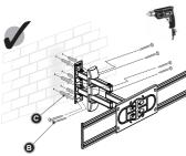
When selecting the position of the TV mount. Ensuring that the mount will be mounted on to a flat surface and is level. Mark the wall where the fixing locations are. Drill the holes using a 10mm masonry bit. Using a hammer knock the the wall plugs (C) provided into the wall. Holding the TV mount start in the one corner screw the provided screws (B) into the wall fixing the opposite corners until the mount is secure onto the wall. Ensure all are tight and secure.
