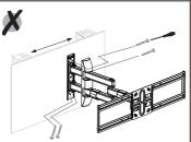
When selecting the position of the TV mount ensure that it is fixed onto a wooden joist or onto a solid wall. Mark the wall where the fixing locations are ensuring that the mount will be mounted on to a flat surface and is level.
