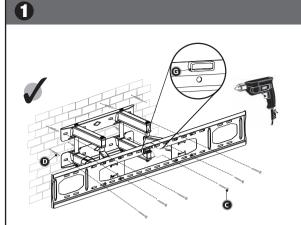
When selecting the position of the TV mount. ensuring that the mount will be mounted on to a flat surface and is level. Mark the wall where the fixing locations are. Drill the holes using a 10mm masonry bit. Using a hammer knock the the wall plugs (D) provided into the wall. Holding the TV mount start in the one corner screw the provided screws (C) into the wall fixing the opposite corners until the mount is secure onto the wall. Ensure all are tight and secure.
