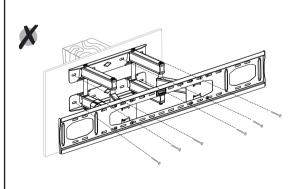
Ensure that the mount is fixed onto a solid surface and not directly onto plaster board.
