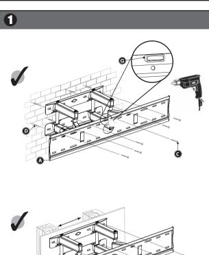
When selecting the position of the TV mount. ensuring that the mount will be mounted on to a flat surface and is level. Mark the wall where the fixing locations are. Drill the holes using a 10mm masonry bit. Using a hammer knock the the wall plugs (D) provided into the wall. Holding the TV mount start in the one corner screw the provided screws (C) into the wall fixing the opposite corners until the mount is secure onto the wall. Ensure all are tight and secure.
