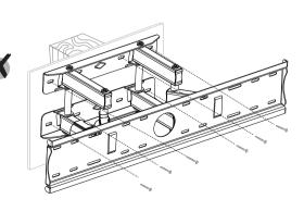
Ensure that the mount is fixed onto a solid surface and not directly onto plaster board.
