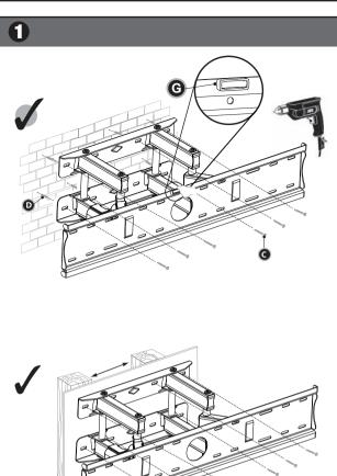
When selecting the position of the TV mount. ensuring that the mount will be mounted on to a flat surface and is level. Mark the wall where the fixing locations are. Drill the holes using a 10mm masonry bit. Using a hammer knock the the wall plugs (D) provided into the wall. Holding the TV mount start in the one corner screw the provided screws (C) into the wall fixing the opposite corners until the mount is secure onto the wall. Ensure all are tight and secure.
