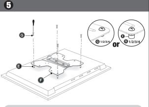
Provided select the appropriate ones to hold the hooks (G) onto the TV. Ensuring that the mounts are facing the the top end of your TV screw the mount onto the TV ensuring not to over-tighten.
