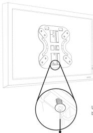
Using a screwdriver tighten the securing bolts onto the mount.
