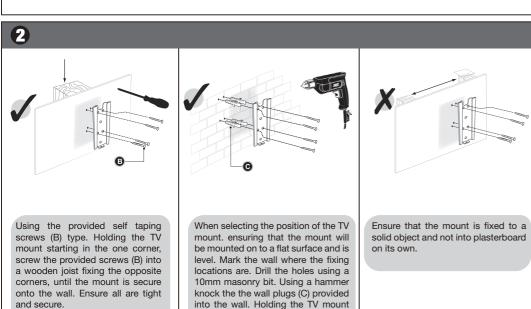
start in the one corner screw the provided screws (B) into the wall fixing the opposite corners until the mount is secure onto the wall. Ensure
