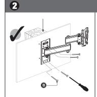
Using the provided self taping screws (B) type. Holding the TV mount starting in the one corner, screw the provided screws (B) into a wooden joist fixing the opposite corners, until the mount is secure onto the wall. Ensure all are tight and secure.
