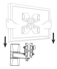
Provided select the appropriate ones to hold the hooks (H) onto the TV. Ensuring that the mounts are facing the the top end of your TV screw the mounts onto the TV ensuring not to over-tighten.
