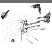
When selecting the position of the TV mount. ensuring that the mount will be mounted on to a flat surface and is level. Mark the wall where the fixing locations are. Drill the holes using a 10mm masonry bit. Using a hammer knock the the wall plugs (C) provided into the wall. Holding the TV mount start in the one corner screw the provided screws (B) into the wall fixing the opposite corners until the mount is secure onto the wall. Ensure all are tight and secure.
