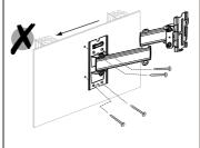
Ensure that the mount is fixed to a solid object and not into plasterboard on its own.
