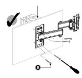
Using the provided self taping screws (B) type. Holding the TV mount starting in the one corner, screw the provided screws (B) into a wooden joist fixing the opposite corners, until the mount is secure onto the wall. Ensure all are tight and secure.
